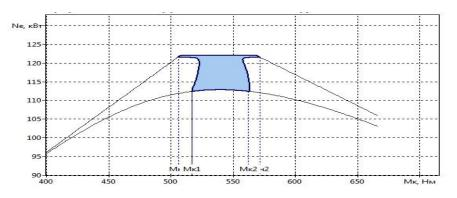
Fig.3. Optimum range for BF06M2012C engine.
