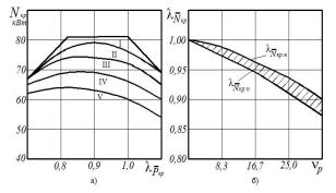
Fig.8. Variation of operation estimations of VT-4S150DMtractor as a function of load rate  $\lambda_{\overline{P}_{\kappa p}}$  and coefficient of its variation  $v_p$  (I –0%; II – 8,3%; III – 16,7%; IV – 25,0%; V – 33,3%): a)- haulage capacity  $\overline{N}_{\kappa p}$ ; b)- probability coefficient
