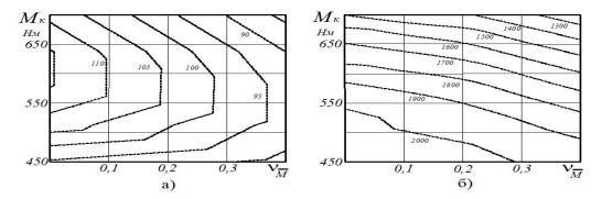
Fig.1. 2D cross section of response surface characterizing alteration of effective power (a) and engine shaft RPM (b) as a function of torque and coefficient of variation.
